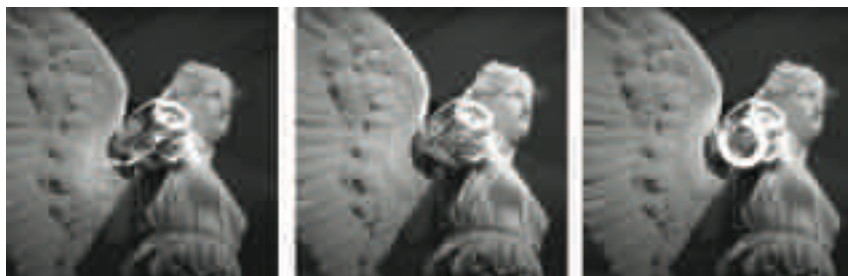
Fig. 4: In the self-guided mode, particles emit from the user-controlled gaze as soon as it enters the collider area of an ROI (left). In the guided mode, the system displays particles over the entirety of the ROI, which has to be confirmed by the user (middle). A dwell timer forms around the sliding puck and has to be completed before the content that is linked to this ROI is delivered (right). As soon as the content is triggered, all particles disappear. Particles are edited and enhanced for visibility in these images.
